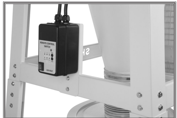
Figure 38. Switch mounted to stand.
